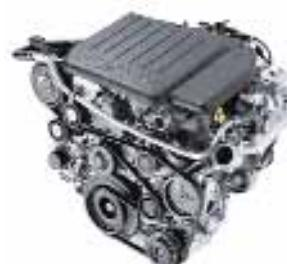
Şekil 2: a. 2.7 lt. Direk Püskürtmeli Diesel Motoru (CRD)
