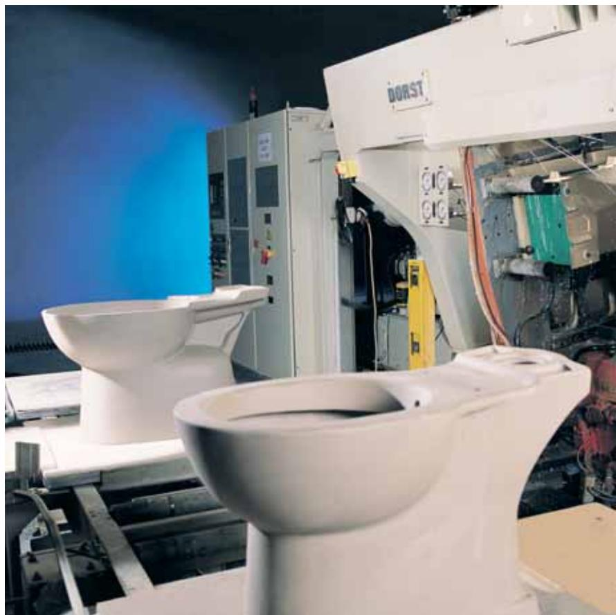
Ware production technology. The remaining 14 % of production is carried out by the classical method using plaster moulds.
